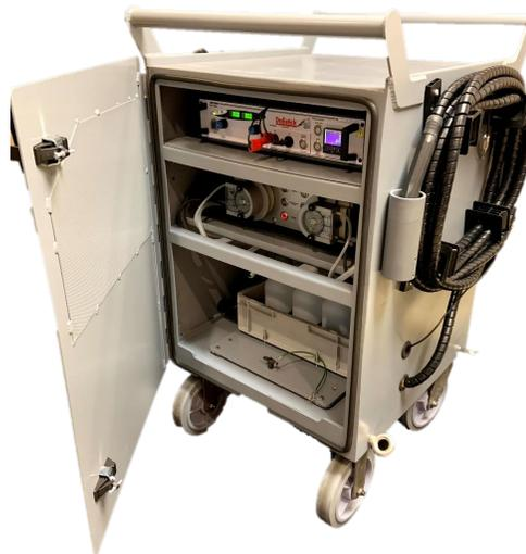
*Corrdesa LLC, GA USA, partnered with Dalic, France to produce the ruggedized, mobile Dalistick® system for ZnNi plating repairs directly on aircraft.*
