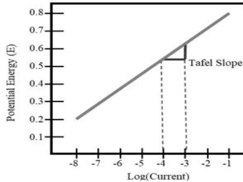
FIGURE C-1. Evans diagram with an arbitrary scale.
