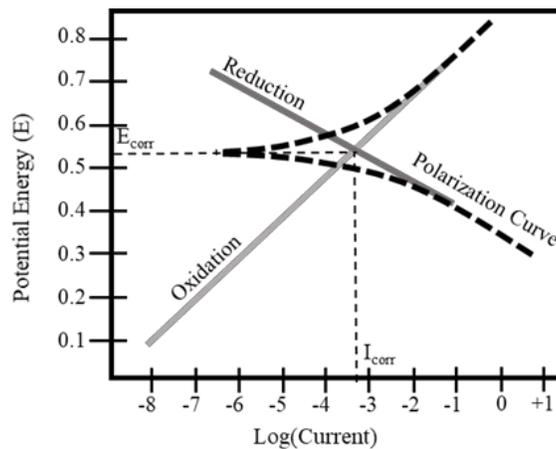
FIGURE C-4. Polarization curve with an Evans Diagram.
