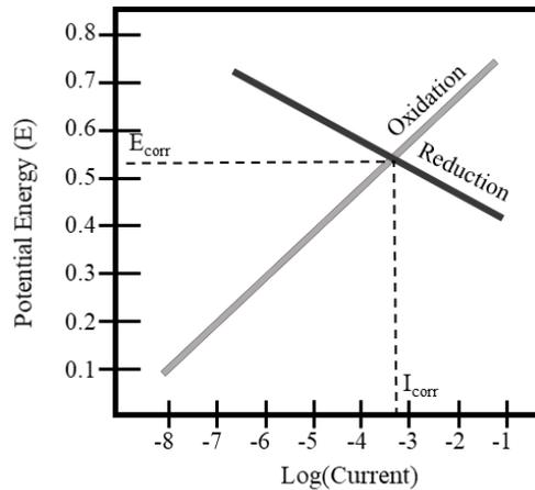
FIGURE C-3. Evans diagram with  $E_{\text{corr}}$  and  $I_{\text{corr}}$ .
