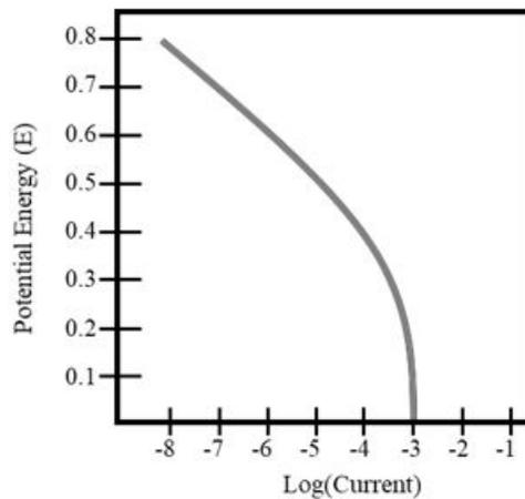
FIGURE C-2. Tafel plot of a diffusion limited system.
