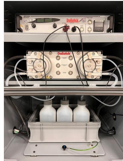
*Corrdesa LLC, GA USA, partnered with Dalic, France to produce the ruggedized, mobile Dalistick® system for ZnNi plating repairs directly on aircraft. Image Courtesy Corrdesa LLC, Distribution A: Approved for public release; distribution is unlimited.*
